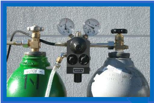
In these cases the work is conducted using locally supplied gas, which is delivered directly to the welding area.
