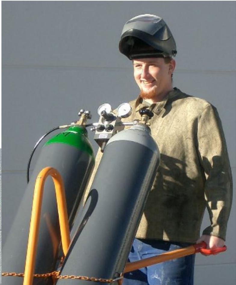
Thanks to this solution only gases need to be stored, and there is no need to use a number of cylinders with pre-mixed gases, which is complicated and expensive. Not to mention the fact that a cylinder with just one gas is usually less expensive than a pre-mix.
