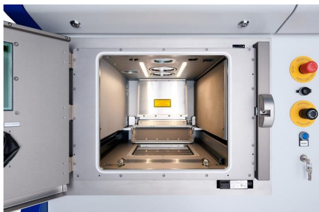
Process chamber of the Selective Laser Melting Machine SLM280 2.0 of SLM Solutions Group AG
