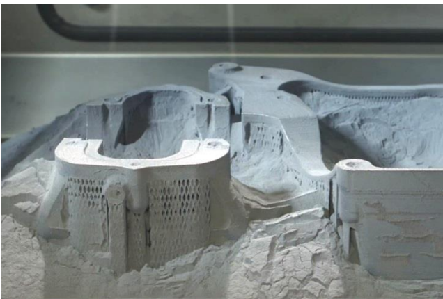
3D-printed components made of metal powder, formed in the process chamber of the Selective Laser Melting Machine SLM500 from SLM Solutions Group AG
