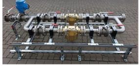
Upon request, a motorised shut-off valve was included on the inlet, to allow complete shut-off. Additionally, manual shut-offs before and after each regulator were included, to allow the evacuation of each line. The design, build and commissioning of the system was undertaken by WITT partner Gustus & Partner GmbH, in cooperation with the customer.
