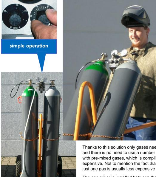
Thanks to this solution only gases need to be stored, and there is no need to use a number of cylinders with pre-mixed gases, which is complicated and expensive. Not to mention the fact that a cylinder with just one gas is usually less expensive than a pre-mix.
