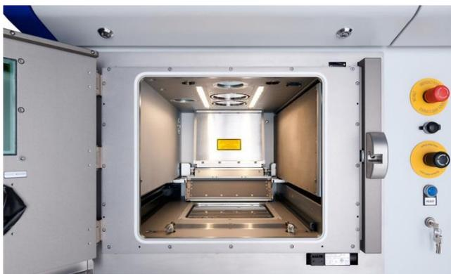
*Process chamber of the Selective Laser Melting Machine SLM280 2.0 of SLM Solutions Group AG*
