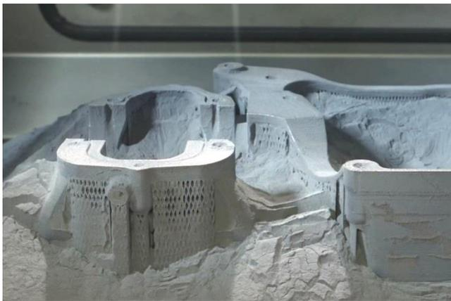
*3D-printed component made of metal powder in the process chamber of the Selective Laser Melting Machine SLM 500 from SLM Solutions Group AG*
