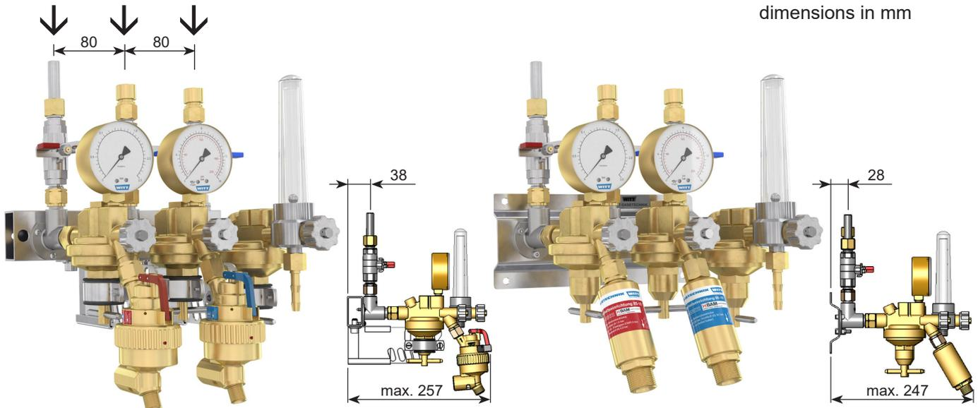
Outlet points easy to use for withdrawal of technical gases. To mount on wall for connection with a central gas supply system (ring line). The compact design is modular expandable and offers a variety of possible combinations.
