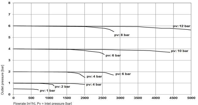
Flowrate [ $m^3/h$ ], Pv = Inlet pressure [bar] 1  $m^3/h$  = 35.3 scfh
