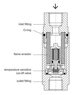
WITT Flashback Arrestors F53N/HHO for reliable protection against dangerous flashbacks at application of hydrogen-oxygen mixtures.
