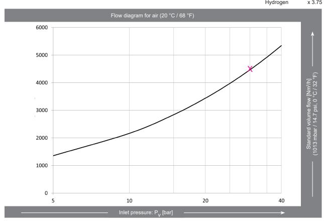
Δp max. = 1 bar in continuous operation
