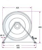
floor fixing or (turned at 180°) ceiling mounting\_
